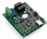
Door Controller RS485
